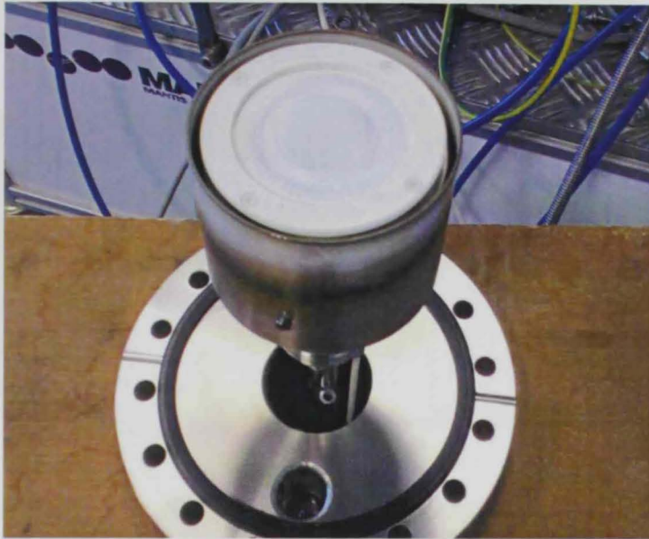
Fig. 11. The magnetron sputter gun with Ag target.
