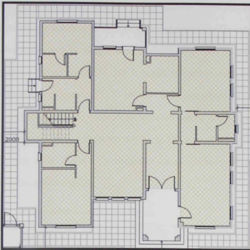
Figure 5.1: Typical Ground Floor Plan for the Five-bedroom Villa
