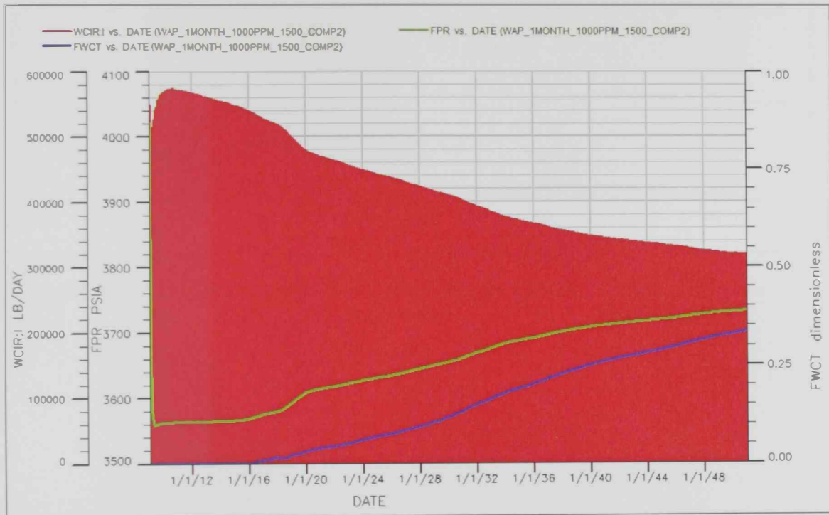
Figure 5.34: WAP injection at 1500 STB/D (1000 ppm, COMP2, 1 month) reservoir performance
