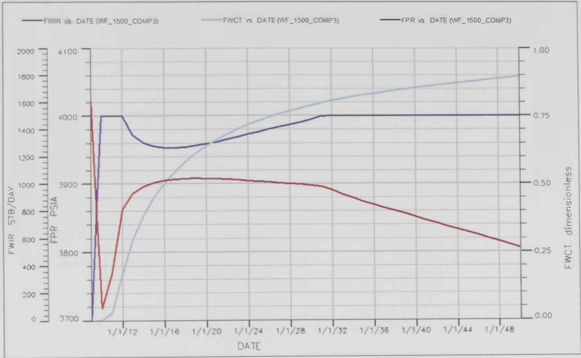
Figure 5.12: Waterflooding injection at 1500 STB/D (COMP3) reservoir performance
