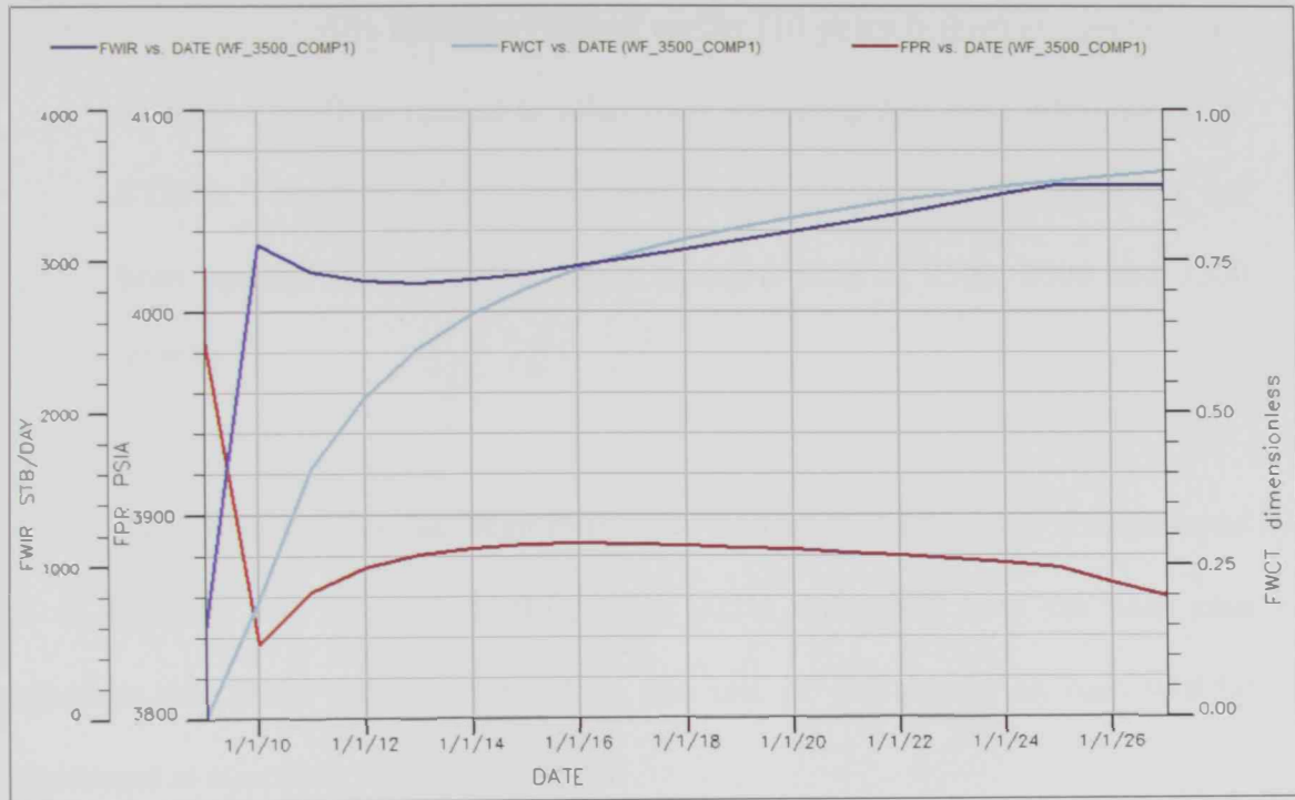
Figure 5.8: Waterflooding injection at 3500 STB/D (COMP1) reservoir performance
