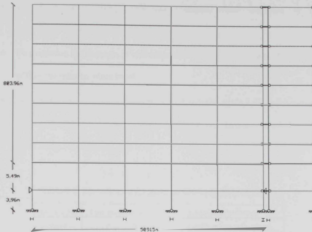
Figure 2.21: OpenSees model of a reference structure studied by Michalis et al. (2006)
