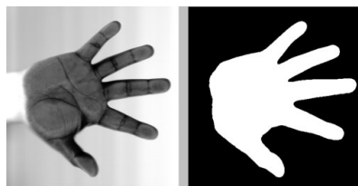
Figure 5: Appearance-based algorithm for Gesture Recognition (Ramirez-Cortes, Gomez-Gil, Sanchez-Perez & Prieto-Castro, 2009)
