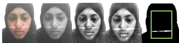
Figure 15: Brightest laser reflection in green box is detected as the user's face
