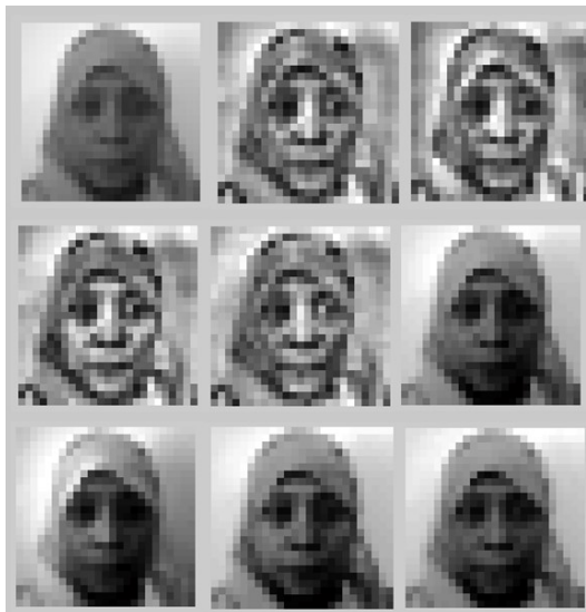
Figure 16: First row left-right: grey scale image, AHE on RGB channels, AHE on R channel; second row left-right: AHE on B channel, AHE on G channel, HE on RGB channels; third row left-right: HE on RGB channels individually
