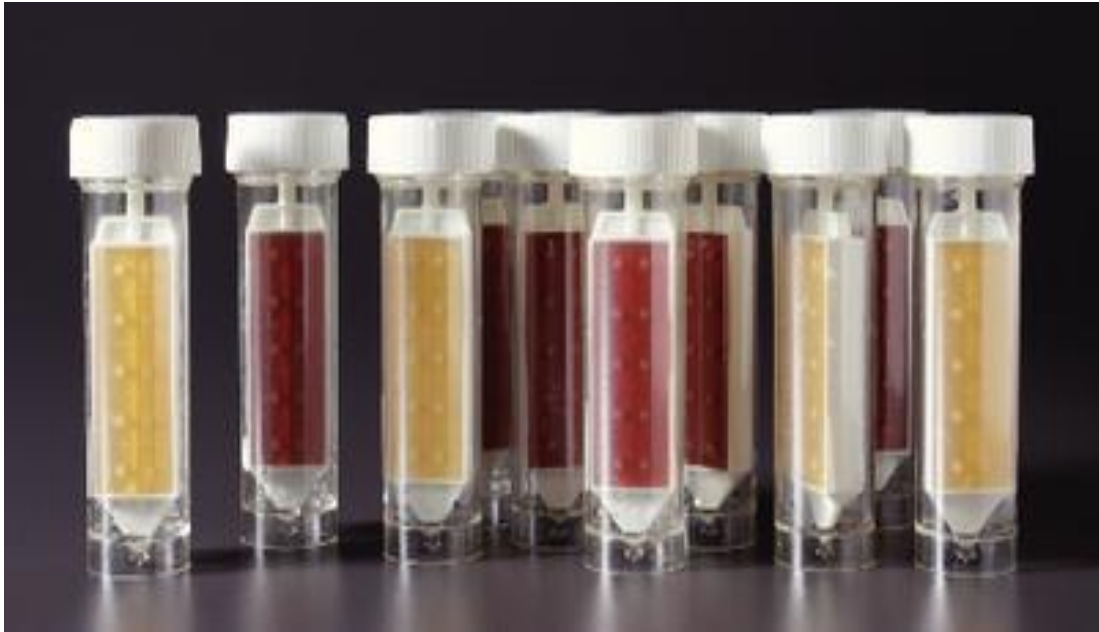
Figure 3.5: HACH Paddle Tester (Cat No. 26109-10) for total aerobic bacteria and total coliform test
