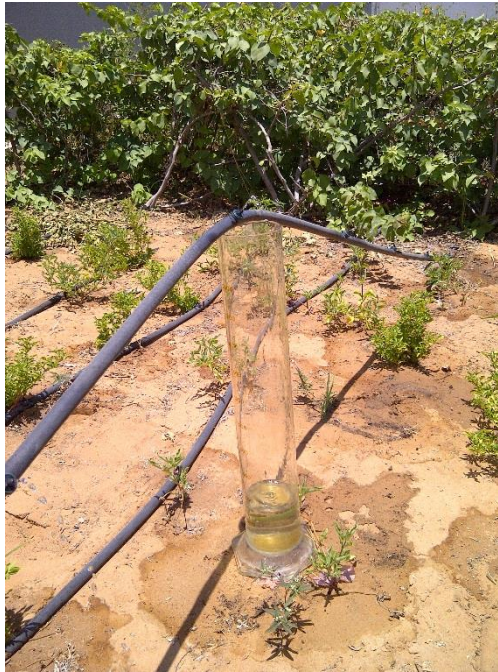
Figure 3.7: Irrigation water demand estimation in urban landscape using a volumetric glass jar and stop watch
