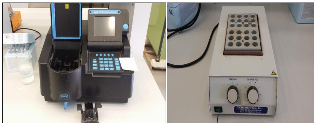
Figure 3.4: DR/4000U Spectrophotometer (left) and a oven to heat COD bottles (right) used in the experiment for COD test (placed in the Environmental Engineering laboratory, UAEU)
