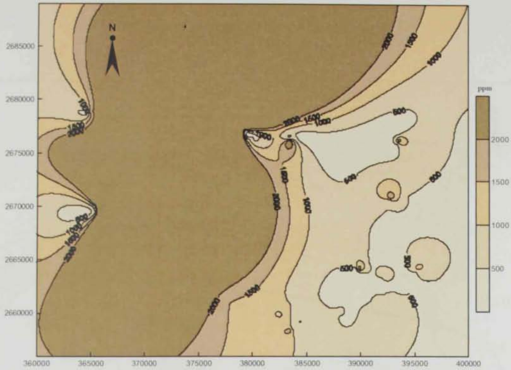
Fig. (5.13) Distribution map of the chloride anion for the Quaternary aquifer in Al Jaww plain.
