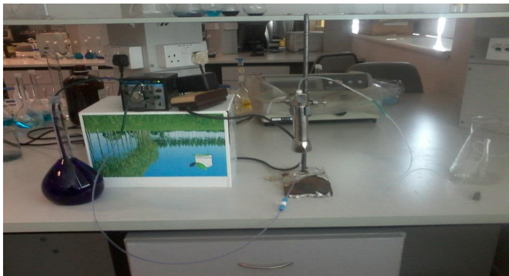
Figure 78: Dynamic adsorption study set-up for 10 ppm Crystal Violet (CV)
