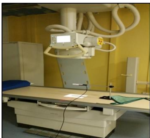
Figure 9: Air kerma measurements setup- (Table Bucky)
