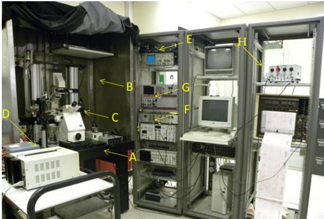
Figure 2.3 The recording system used for video edge detection and \text{Ca}^{2+} imaging experiments: The system includes an anti-vibration table (A), a Faraday cage (B), an inverted microscope (C), a cell superfusion system (D) with a temperature control system (E), a video edge motion detector (F), a microfluorescence photometry system (G) and an electrical stimulator (H).
