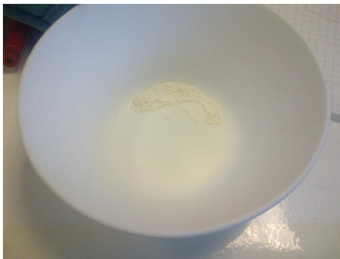
Fig. 2.10 The rock sample with no residue (looks like dry salt) after 3 times repetition of HF and HNO 3 addition.
