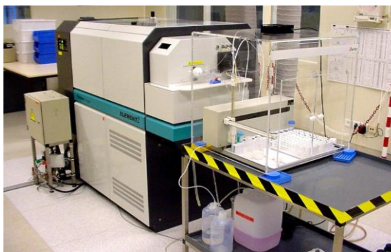
Fig. 2.9 The ICP-MS instrument used for uranium and thorium mass concentrations at the Technical University of Denmark (Center for Nuclear Technologies, Risø campus).
