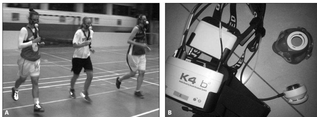
Fig. 5: A) The BEEP TEST performed by a participant. B) The K4b2 measurement system (Cosmed, Italy). Source: authors' own photographs
