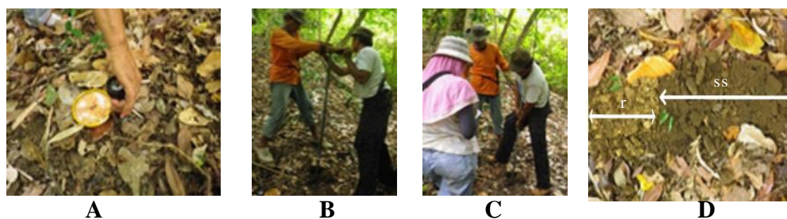
Figure 2. (A.) Direct measurements of soil temperature, moisture, and pH; (B.) Soil coring at the site; (C.) extracted soil sample from the pit; (D.) SS is soil solum; r is regolith.
