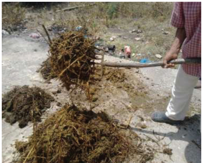
Figure 2: Coning and quartering in progress as part of the process of creating a final sample. The biomass here is cattle manure
