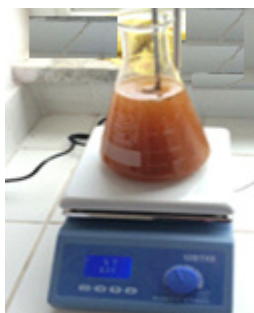
Figure 2: Hot water extraction.
