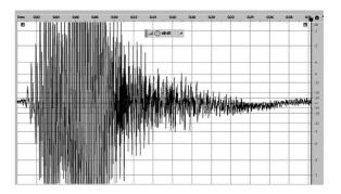
Figure 7. Noise decay from 0 dB to -24 dB in 200 ms.
