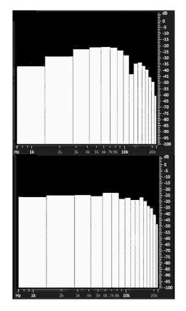
Figure 10. Frequency response to white noise pointing across the room to the space between S1 and S6 in Figure 6 (top), and S1 and S2 (bottom)
