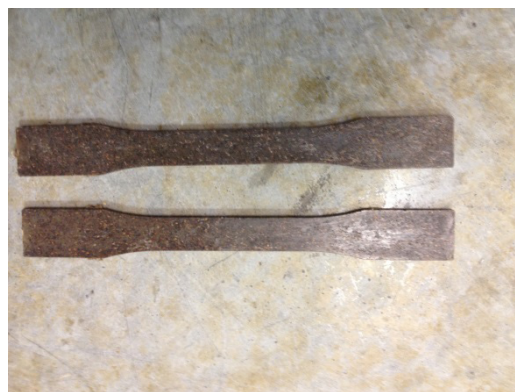
Figure 1. WPC sample test according to ASTM 638-03.
