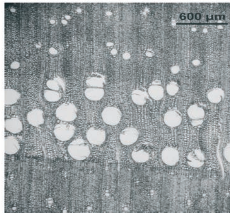
Fig. 6. Optimised steam hydro thermolysis of Ash (cross section), without damages of wood structure
