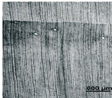
Fig. 2b. Liquid full hydro thermolysed treated Norway spruce (cross section), with larger annual rings and a gradual transition from earlywood to latewood. No tangential cracks in the latewood section are visible
