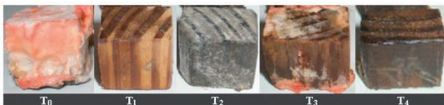
Figure 5. View on the test tubes after 3 months of culture with Pycnoporus sanguineus . Abundant colonization in the pinewood without impregnation (T 0 ).
