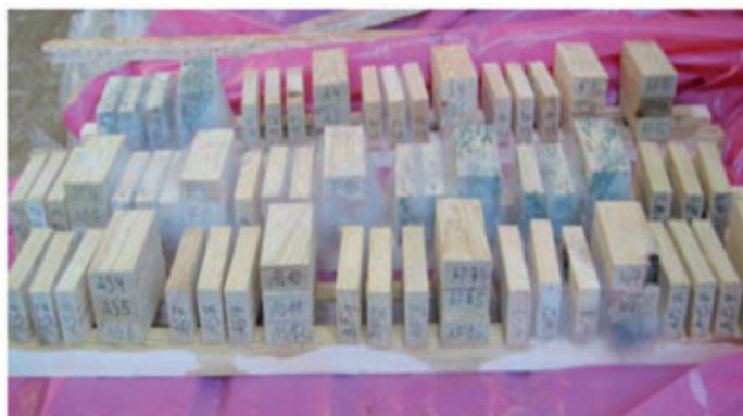
Figure 4. Small size test specimens used in screening fungi-static effect of environmentally compliant agents
