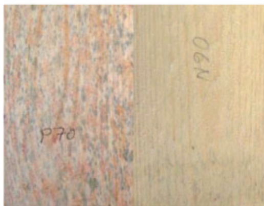
Figure 2. Development of mould on ISPM NO 15 heat-treated pine sapwood (left) and untreated control (right) after 7 days under plastic cover
