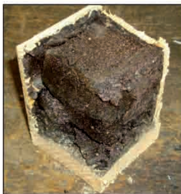
Figure 7. Appearance of plywood box as opened after 8 months exposure to wet winter weather. Note that the tannin-based foam is still in good condition.
