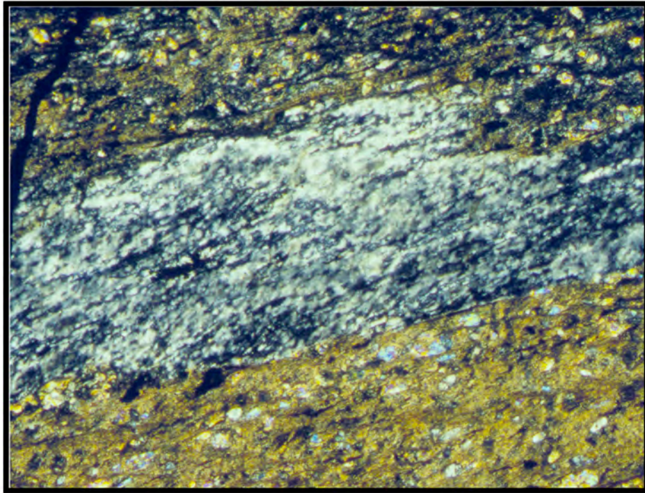
Figure 3.4 - Tourmaline porphyroclasts in mylonite. Dark green crystals have c-axis perpendicular to plane of view; light green = parallel with lineation & pov.
