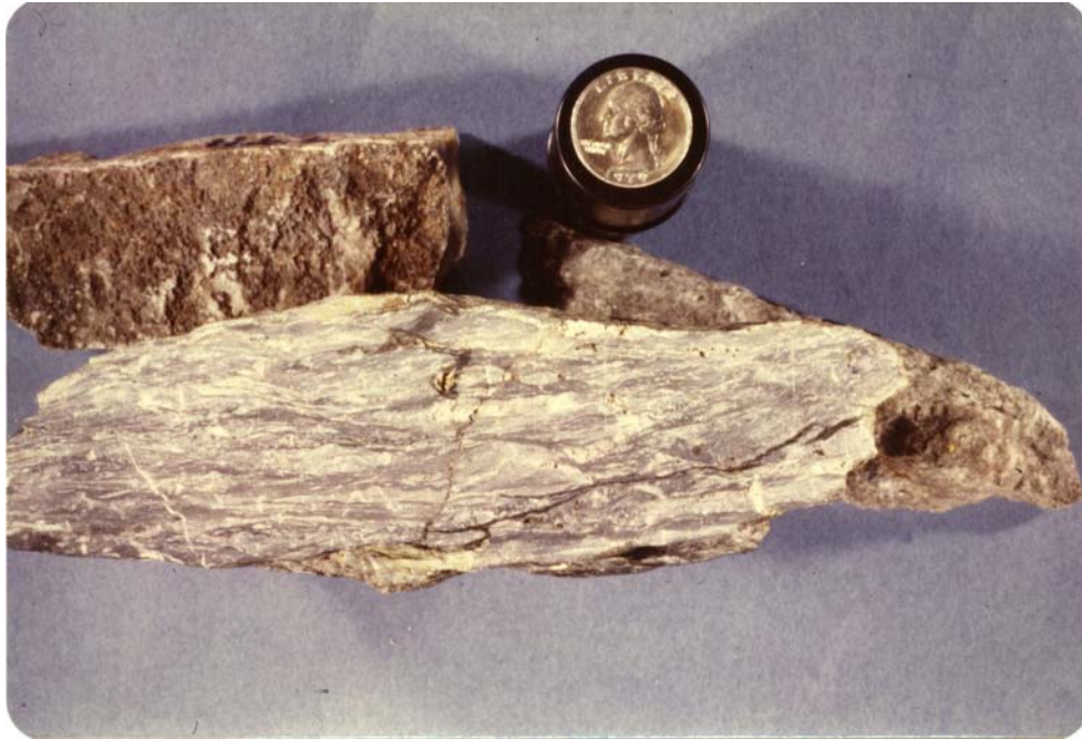
Figure 55a: Photograph of hand specimen of fault rock collected from locality 9+6 on figure 23. Note folded to highly dismembered quartz veins with cleavage axial surface to folds. A weak lineation is apparent on the cleavage surface.
