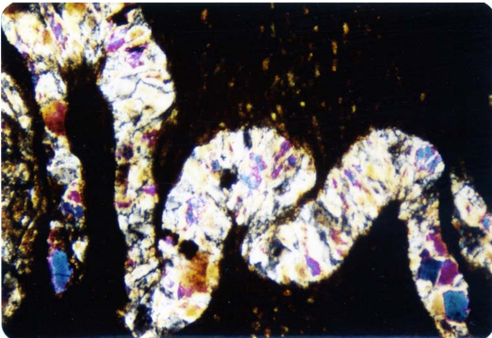
Figure 62: Photomicrograph of a relatively wide tightly folded and partially dismembered quartz (section very thick) vein. Vein initially oriented approximately perpendicular to present foliation. Note the lack of polygonal grains and sutured appearance of grain boundaries. The elongate shape of the grains define convergent fans within the veins. The well developed foliation within the argillite matrix is axial surface to the folds of the vein and form divergent fans in the hinge areas. (40x magnification, 3.64 mm field of view).
