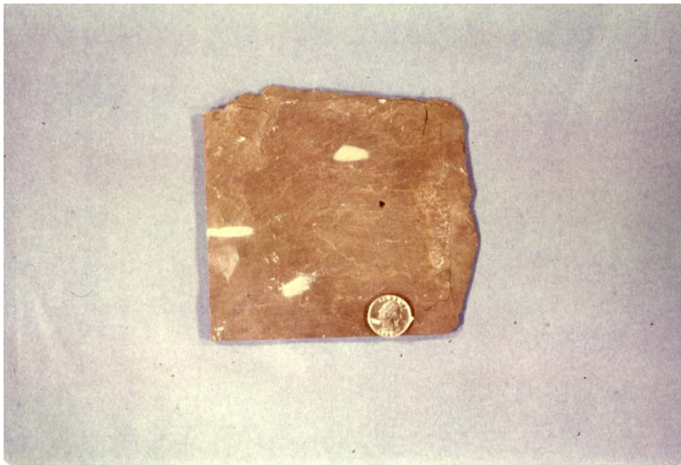
Figure 42: Ellipsoidal reduction spot on cleavage surface.
