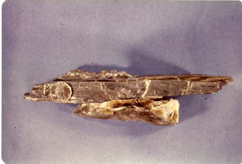
Figure 44: Deformed fibrous vein quartz. Deformation may be associated with late stages of slaty cleavage development.
