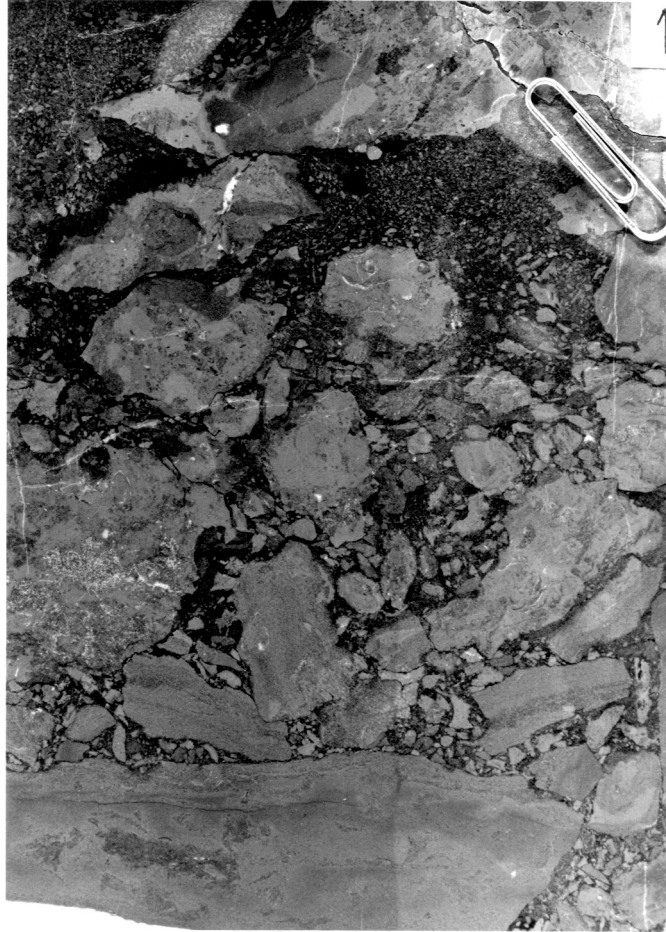
Fig. 4.5.- Polished and etched slab of dolostone showing solution-collapse breccia. The matrix contains dedolomite. Providence Island Section (loose fragment). Arrow indicates "top" of the fragment as it was found.
