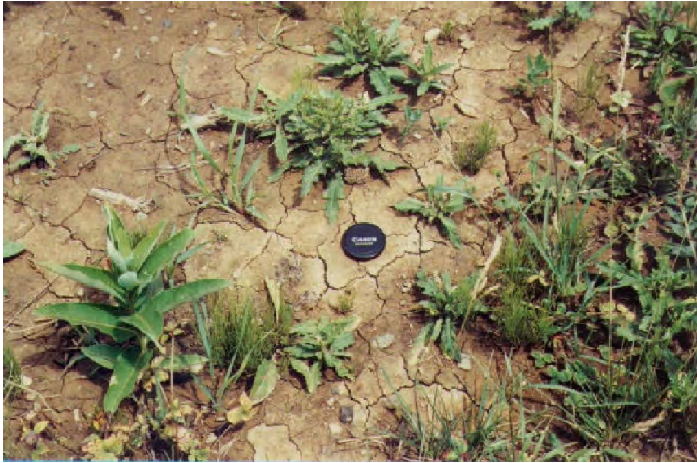
Figure 4.10 Example of clayey soil and mudcracks overlying tile drain 2 (TD2). Photograph taken on July 5th, 1999, less than 24 hours since 8.81 cm of rain fell.
