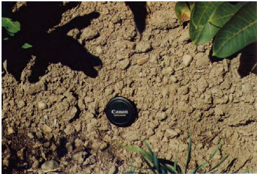
Figure 4.11 Example of gravel and sandy soil overlying tile drain 4 (TD4). Photograph taken on July 5th, 1999, less than 24 hours since 8.81 cm of rain fell.
