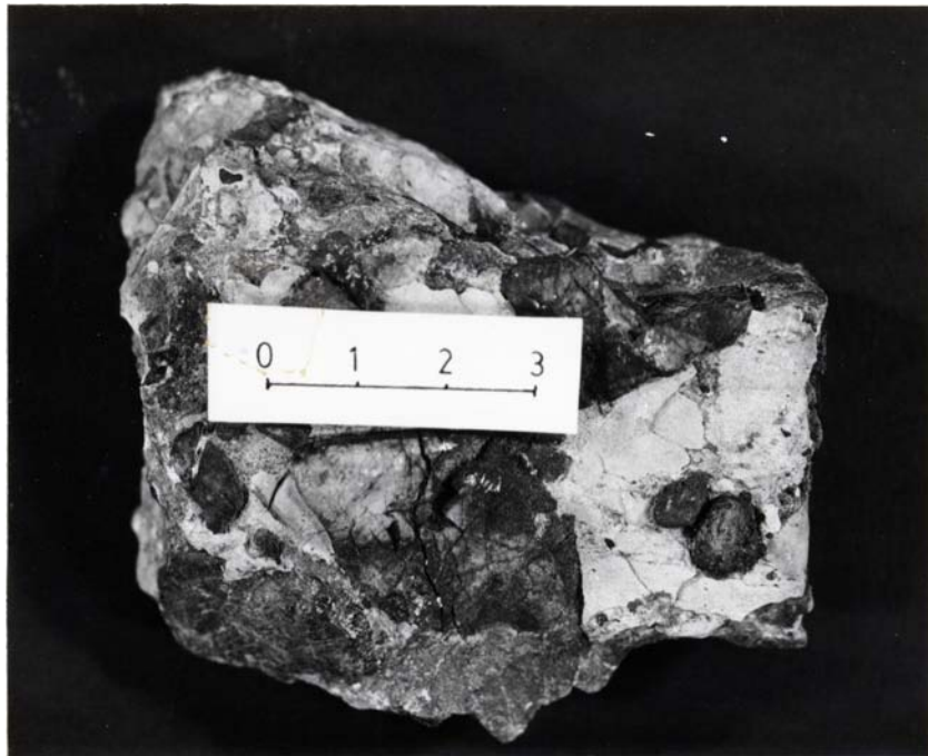
Figure 29. Phosphate pebble conglomerate in the Crossroad Mbr. of the Poultney Fm. This horizon is distinctive but very localized, and the origin of the phosphatic pebbles is not known. The scale bar is in centimeters.
