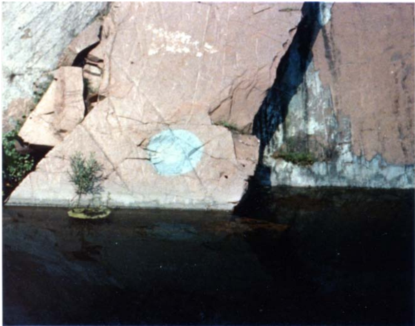
Figure 63. Color change in the Indian River slate. The diameter of the circle is approximately one meter.
