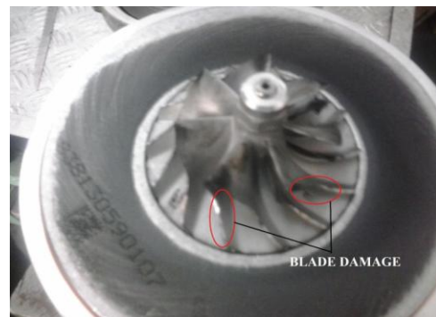
Fig. 1: Damage of Material
