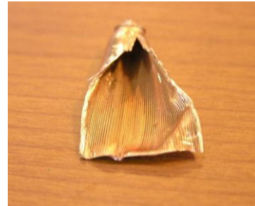
Fig. 1.2: Grooved Wick Type
