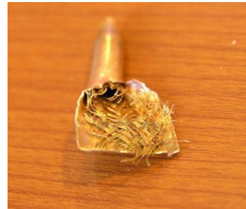
Fig. 1.3: Metal Mesh (Felt) Wick Type
