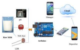
Fig. 1: System Architecture
