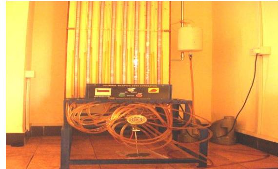
Fig. 2 Journal bearing test rig
