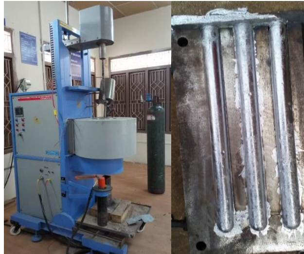
Figure 5: Stir casting machine and die with three finger composite piece.
