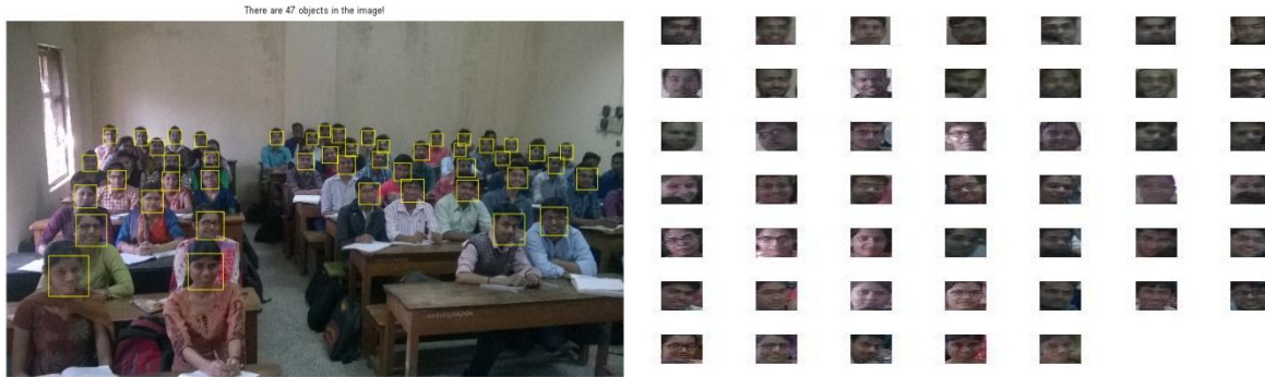
Fig: 5. Detected face of students in live class-room by using Viola-Jones algorithm method.
