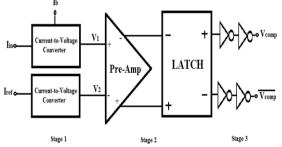
Fig.4. Block diagram of proposed current comparator
