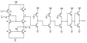
Fig.1. Schematic of Wilson's current mirror comparator
