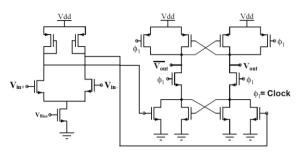
*Fig.3.* Voltage comparison stage: Preamplifier and Dynamic Latch
