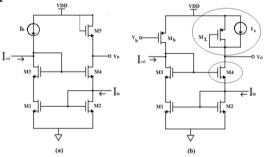
**Fig.2.** (a)Circuit diagram of existing Wilson's current mirror comparator (b) Modifications made in Wilson's current mirror comparator
