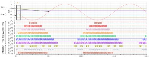
Fig.9. Simulated input and out waveform of 1 GSPS 3-bit ADC employing the proposed comparator
