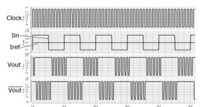
Fig.6. Output response of the comparator for 1µA input difference and 250 MHz input frequency
