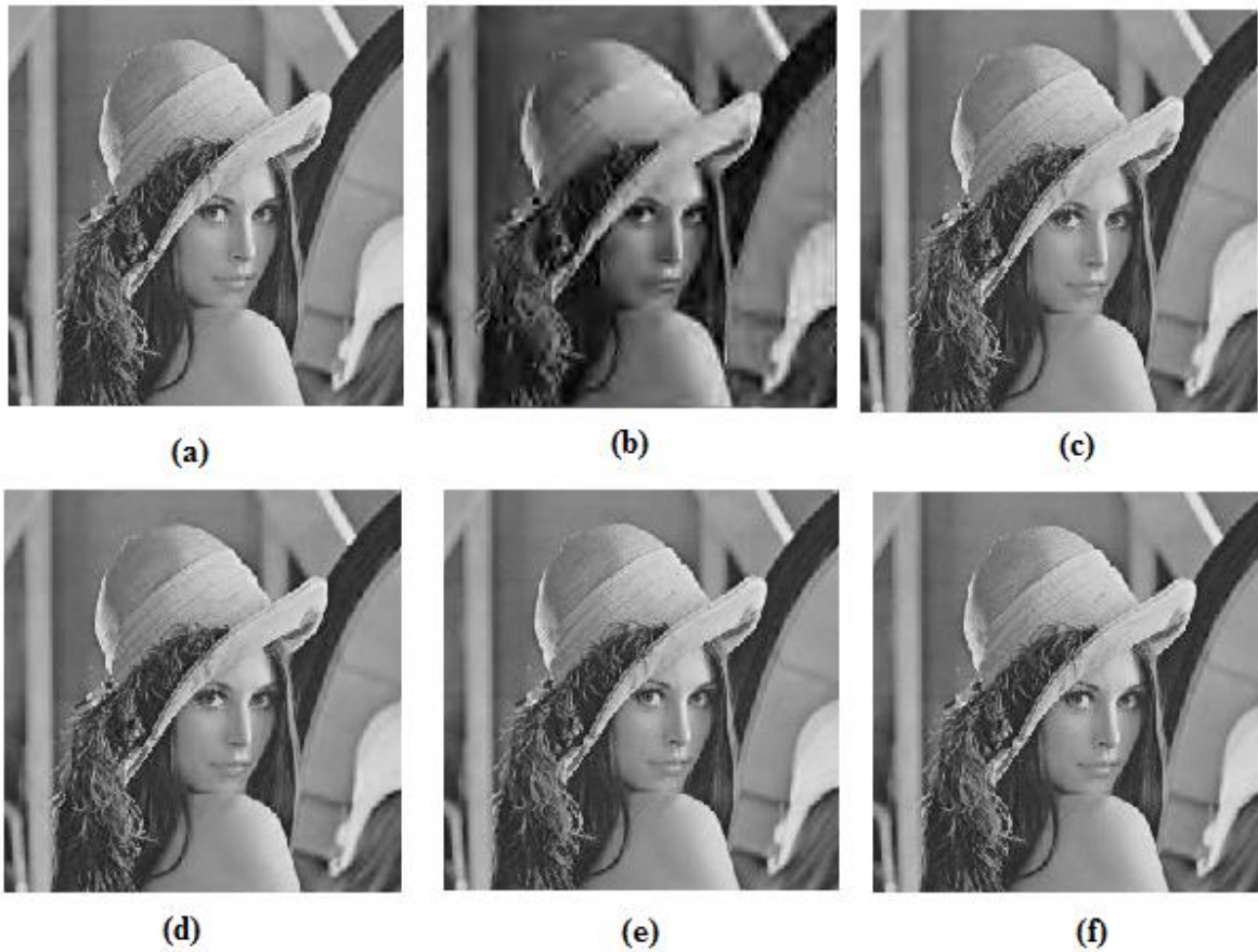
Fig.7 (a) original Lena image is compressed by using (b)EZTW; (c)SPIHT; (d)SPECK; (e)WDR; (f)ASWDR.
