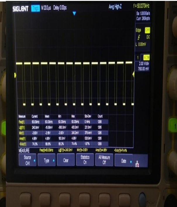
Fig.9. Output With duty cycle 74.4%
