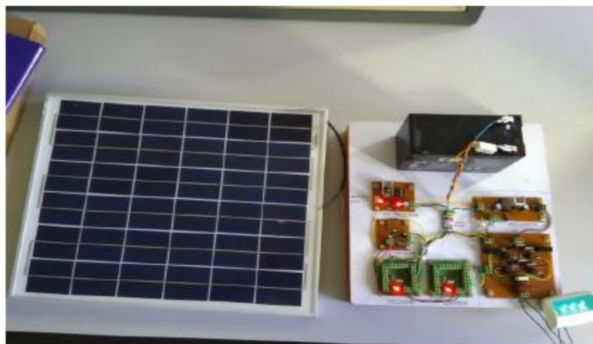
Fig.11 hardware model of SBI with Solar Panel
