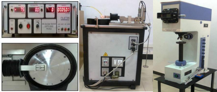
Figure 1: Machine set up for dry wear test and Vickers hardness test
