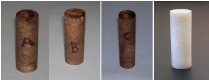
Figure 2: Specimens for Pin on disk Test and Vickers hardness Test.
