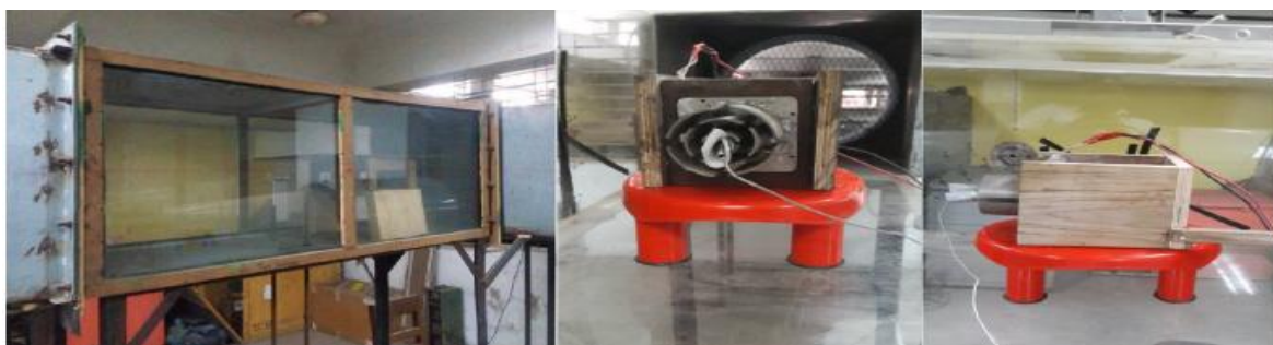
Figure 11: Setup of fin in subsonic wind tunnel for force convection.
