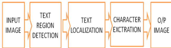
Fig. 3: Basic Block Diagram for Edge Based Text Extraction.
