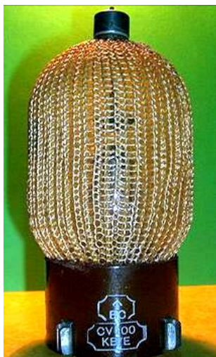
Fig. 6. General view of the powerful trigatron type CV100 [11]
