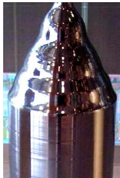
Fig. 12. General view of monocrystalline silicon grown in vacuum by technologists in materials science [18]
