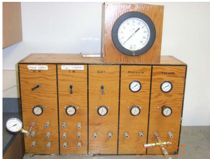
Figure 3.13: Pressure board for Hydraulic conductivity test
