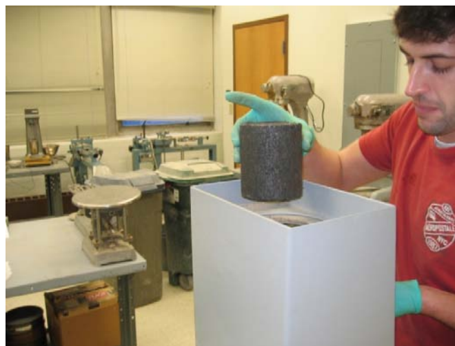
Figure 3.11: Removal of compacted specimen from mold using Jack
