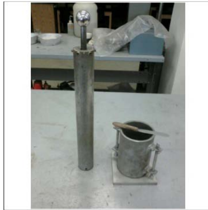
Figure 3.10: Compaction mold with removable collar and Rammer
