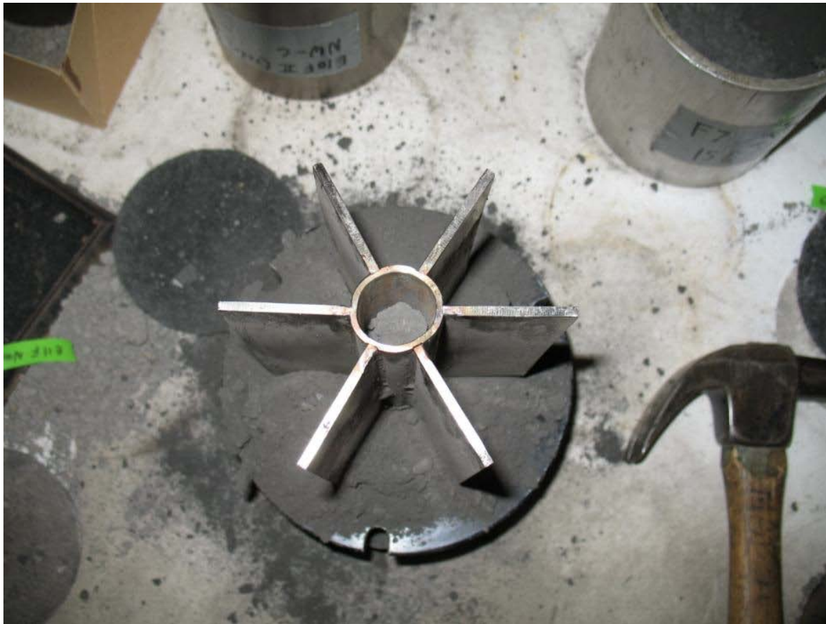
Figure 3.29: Tool completely inserted into the sample
