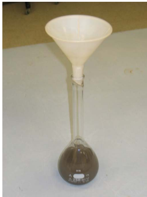
Figure 3.6: Water Pycnometer and the sample for Specific gravity Test
