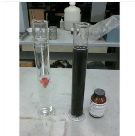
Figure 3.9: Hydrometer analysis with two 1000 ml flasks
