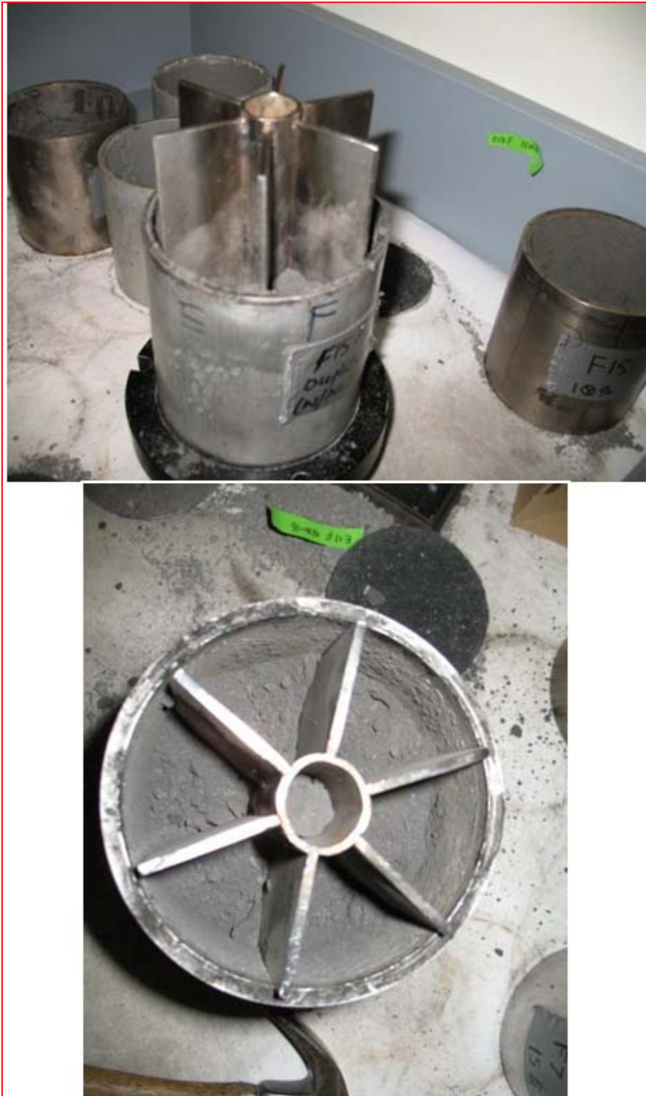
Figure 3.28: Sequence of excavation with tool for particle tracking experiments
