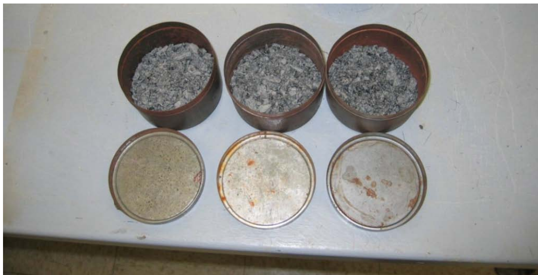
Figure 3.5: Containers and coal refuse sample for Moisture content test
