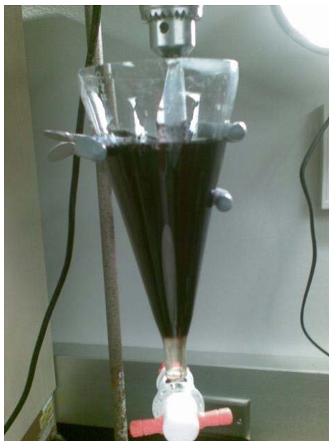
Figure 3.34: Funnel with organic liquid to characterize coal refuse
