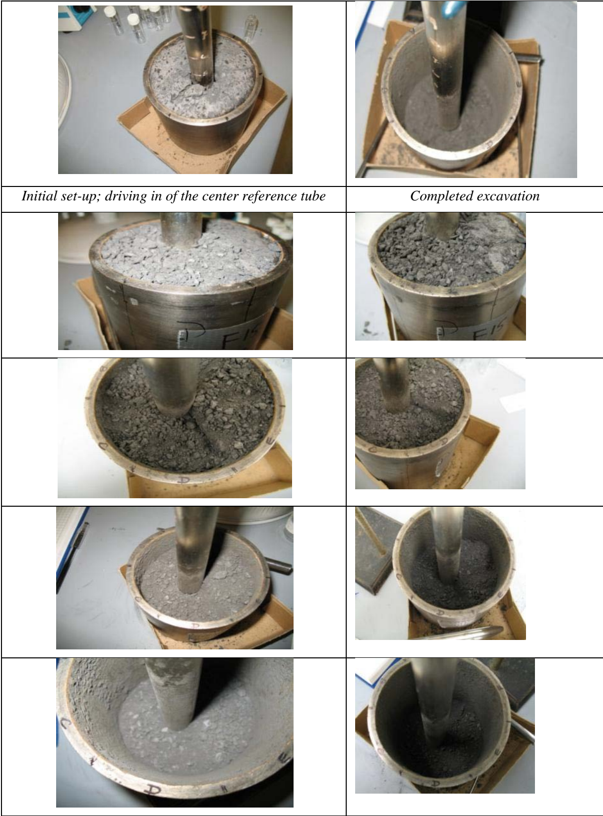
Figure 3.27: Sequence of excavation without tool for particle tracking experiment
