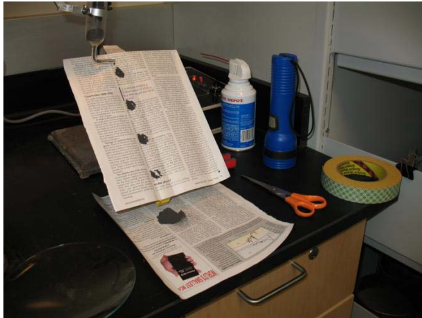
Figure 3.35: Magnetic separation for coal refuse characterization
