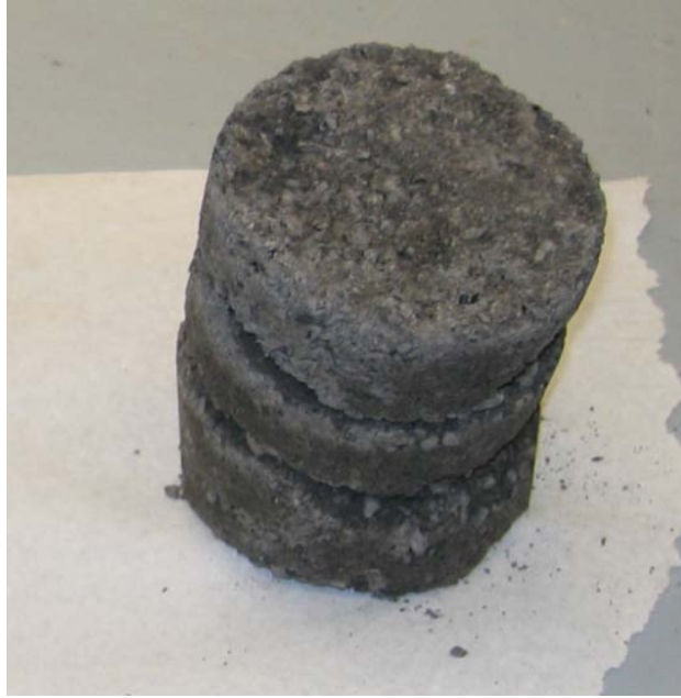
Figure 3.12: Layers of compaction mold specimen for moisture content
