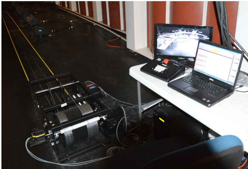
Figure 44: Cable running to winch & computers controlling Automation
