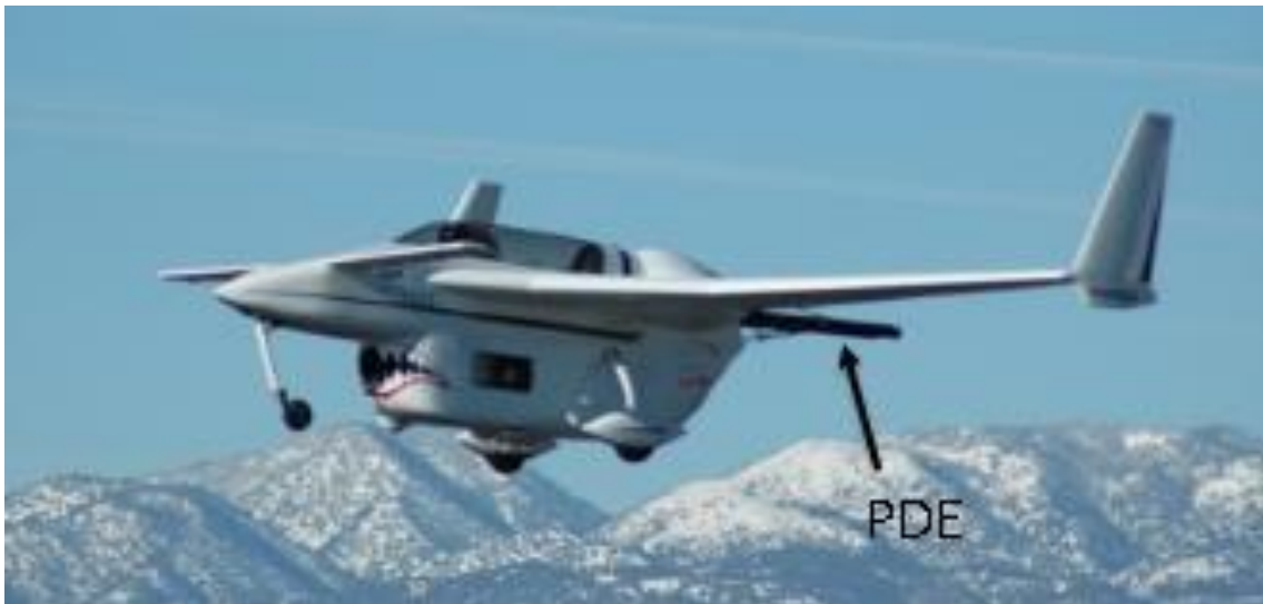
Figure 1: Modified Rutan Long-EZ with PDE during January 31, 2008 test flight. Photo courtesy of Air Force Research Lab.
