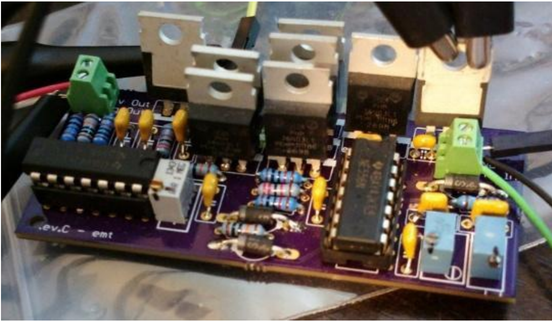
Figure 17: Assembled PWM circuit board during QC testing.
