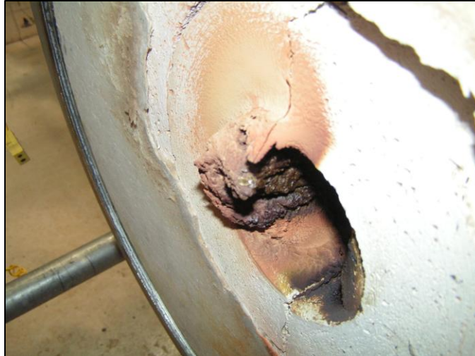
Figure 5.22. Image of transition piece still attached to aerothermal test section displaying large structure of deposition build up.
