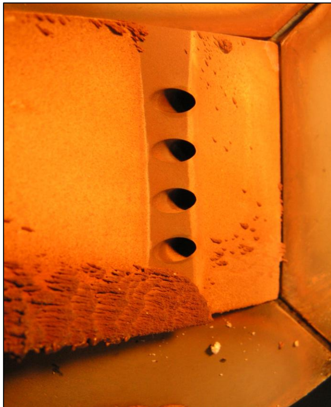
Figure 5.16. Top view of deposition at mainstream temperature of 2315°F on a 20° angle test article at M=1.0 for a 6-hour test.
