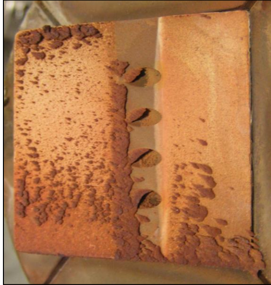
Figure 5.12. Top view of deposition at mainstream temperature of 2315°F on a 20° angle test article at M=0.0 .
