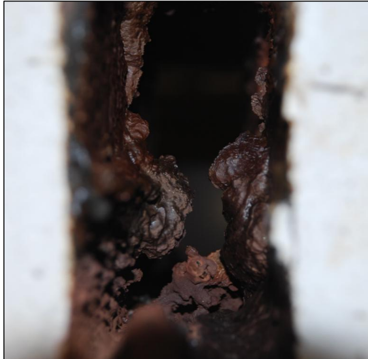
Figure 5.24. Image of deposit structure on transition piece after removal from aerothermal test section.
