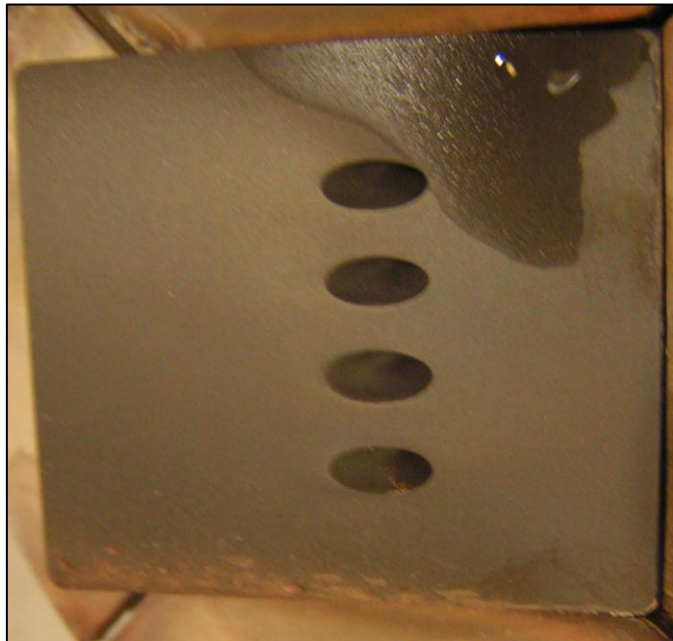
Figure 5.20. Top view of deposition at mainstream temperature of 2315°F on a 20° angle test article at M=1.0 without thermal barrier coating.
