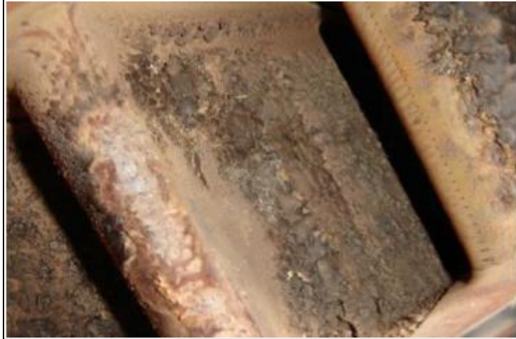
Figure 1.3. Film-cooled turbine vane covered by particulate matter[3].
