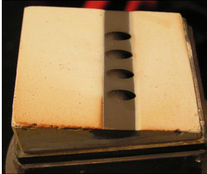
Figure 5.5. Side view of deposition at mainstream temperature of 2200°F on a 10° angle test article at M=1.0.
