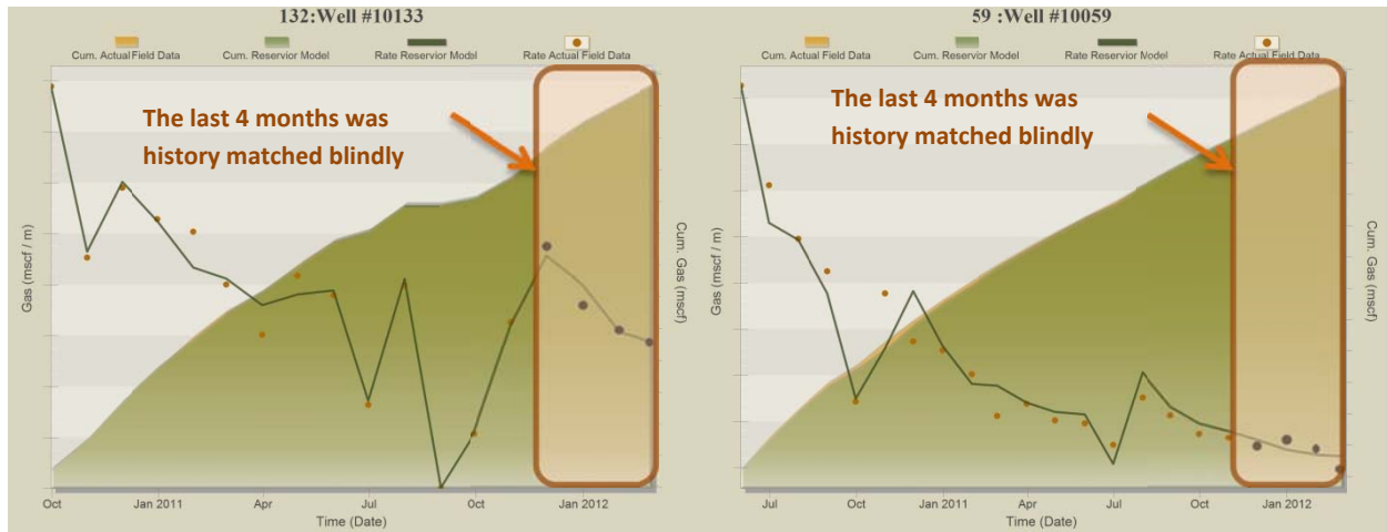
Figure 7.2: The AI-Based model prediction for Well # 10133 and Well # 10059- The last four months was blindly history matched.
