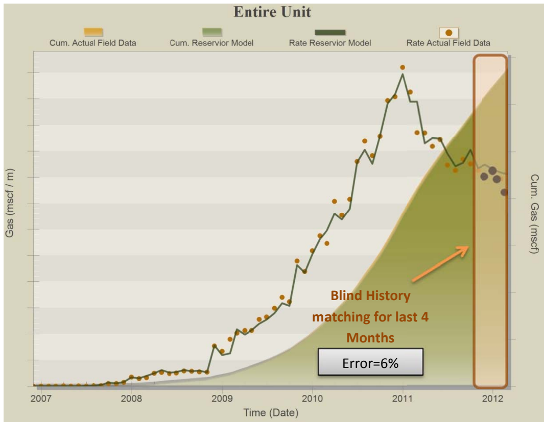
Figure 7.1: The AI-Based Prediction for the Entire Field- the Last Four Months were history matched blindly.
