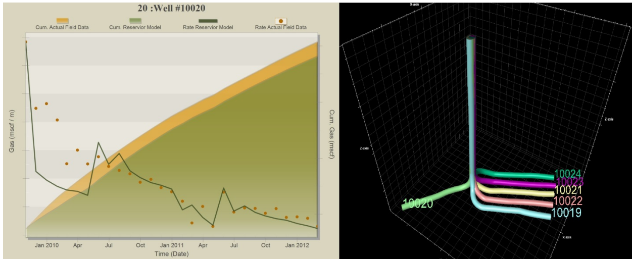
Figure 6.9: The History Matching Result of Well # 10020 after adding the Effect of Offset Well- The Right Plot Shows that This Well is not sharing the drainage area.
