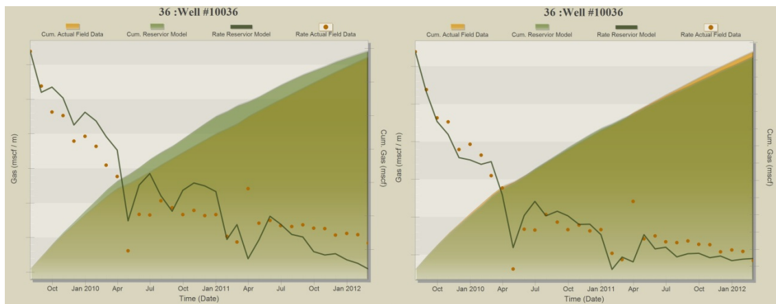
Figure 6.7: History Matching Results for Well # 10036 in Base Model (Left Plot) and Offset Well Model (Right Plot)
