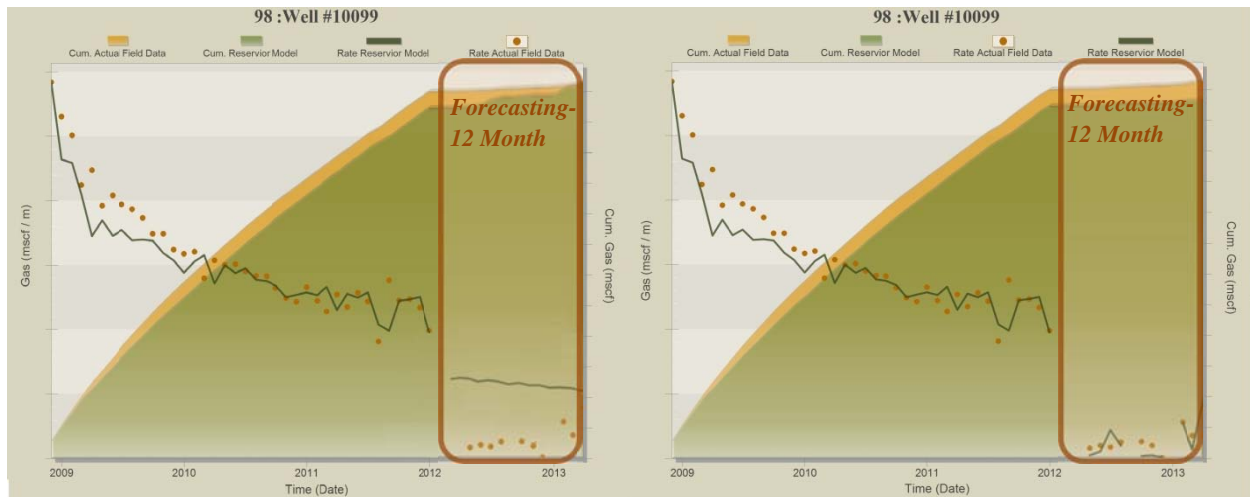
Figure 7.7: The History Matching and Forecasting Result for Well # 10099 before (Left Plot) and after imposing the operational constraints.
