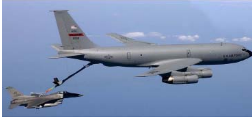
Figure 1.4: KC-135 tanker refuels an F-16 Fighting Falcon using the boom system [63]
