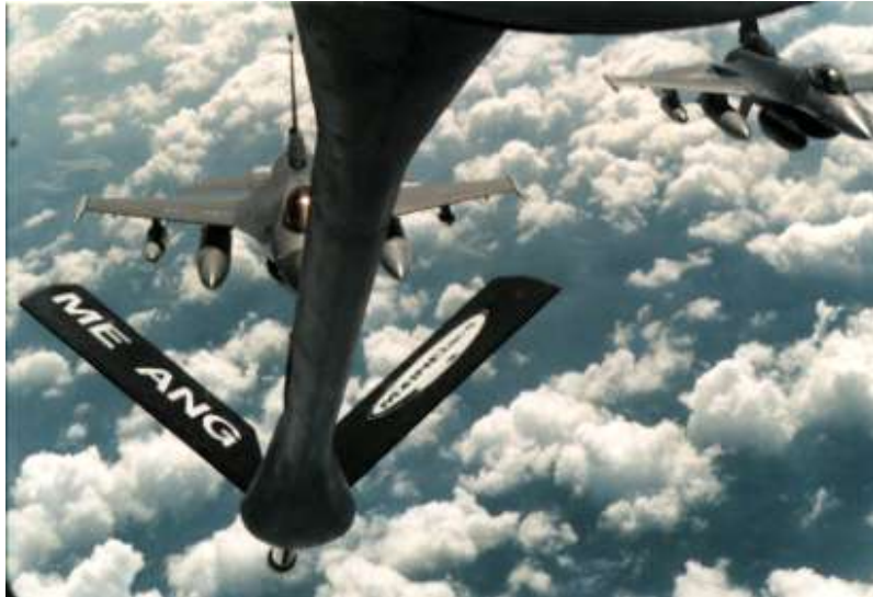
Figure 1.2: The “V” shaped wings of the boom [64]
