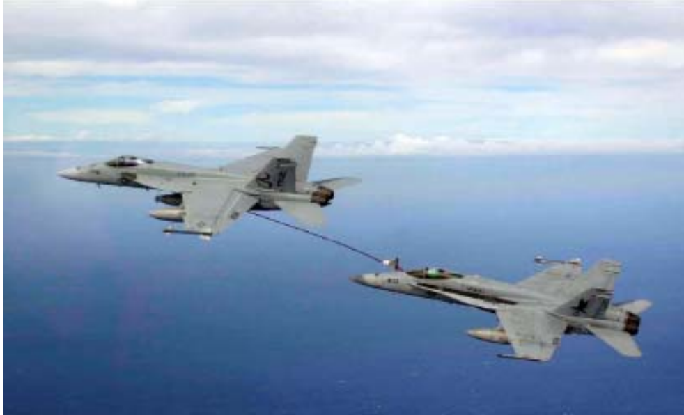
Figure 1.6: F/A-18E Super Hornet performs an in flight refueling evolution with an F/A-18C Hornet using the probe and drogue technique [65]
