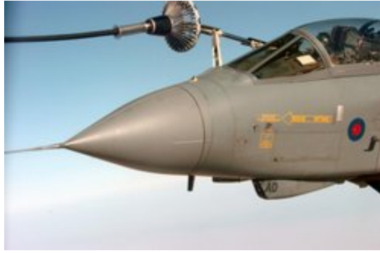
Figure 1.5: Tornado GR4 with probe attached to the drogue of a tanker [1]
