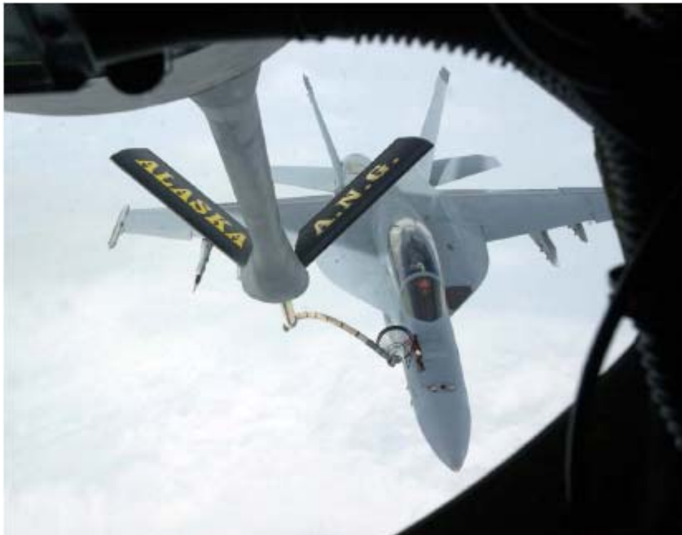
Figure 1.7: Navy F/A-18F Super Hornet is refueled by a KC-135R Stratotanker using a boom-drogue adapter [63]
