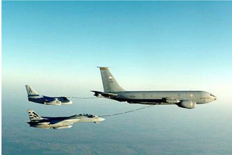
Figure 1.8: A multi point refueling system [66]
