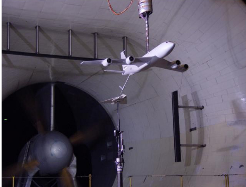
Figure 3.11: Wind tunnel test
