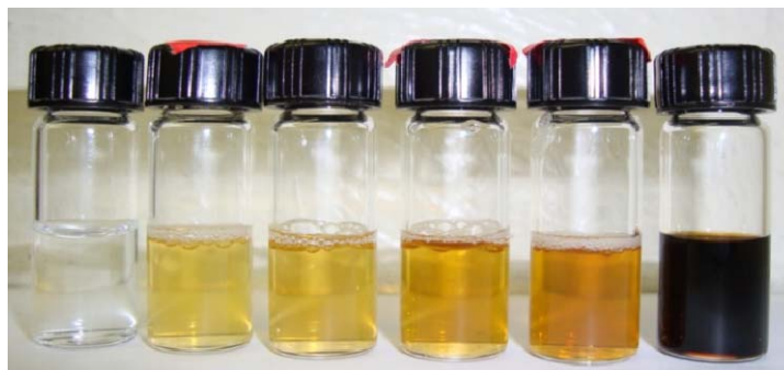
Figure 2-4. From left to right: Water, P 123 coated SPIONs, P 85 coated SPIONs, F 127 coated SPIONs, F 108 coated SPIONs, oleic acid coated SPIONs. All pluronic-SPIONs as aqueous dispersions at the same concentration; oleic acid-SPIONs in toluene.
