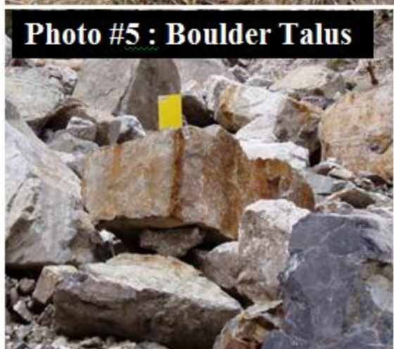
Figure 1: Photographic examples of surface material types available in CRSP (Andrews 2012)
