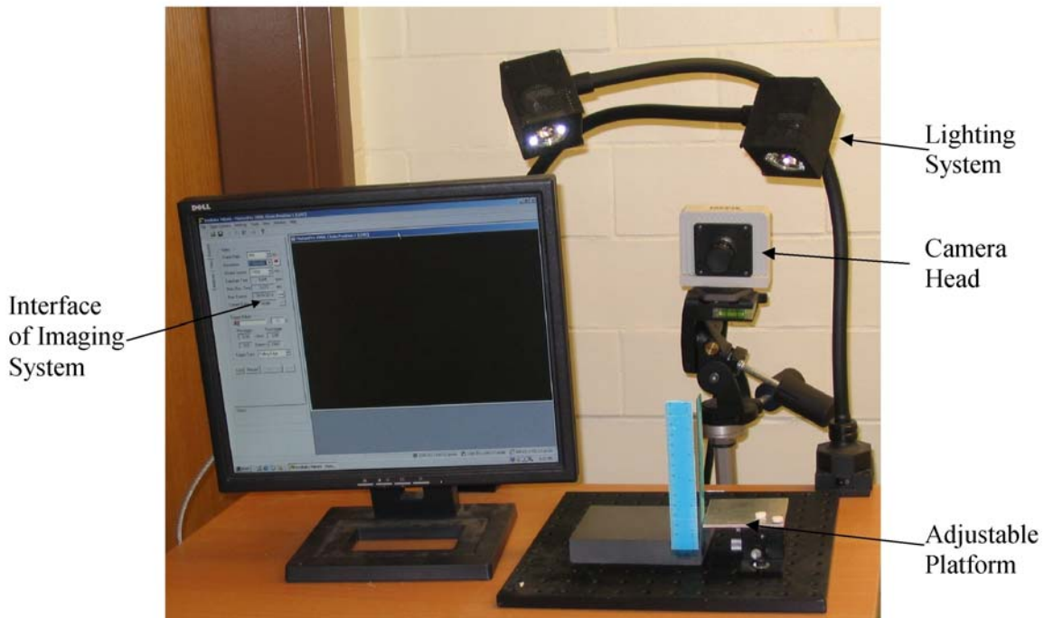
Figure 3.1 Schematic diagram of the high-speed digital imaging system
