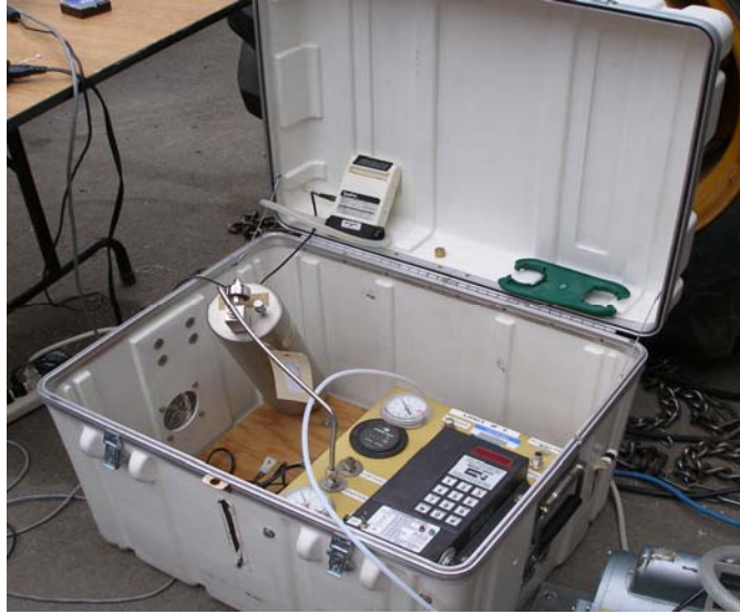
Figure 3.14 DRI pressurized VOC sampling system
