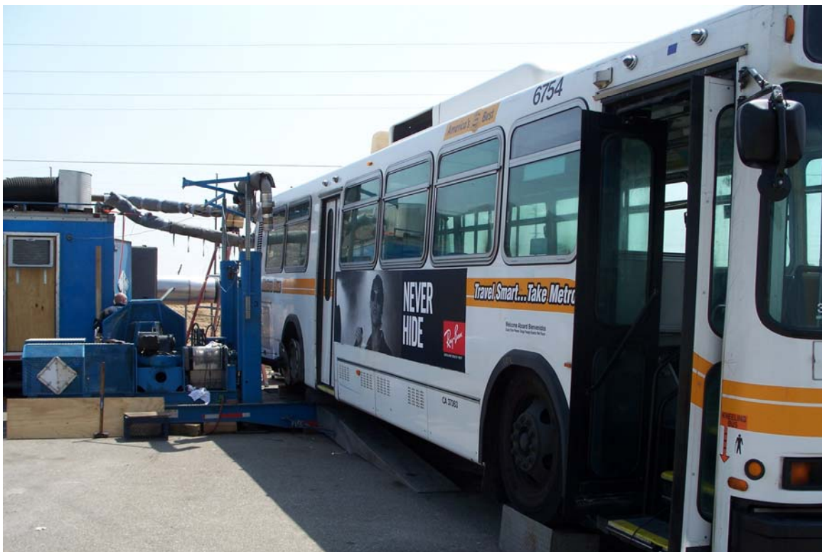
Figure 4.2 Test vehicle mounted on the chassis dynamometer
