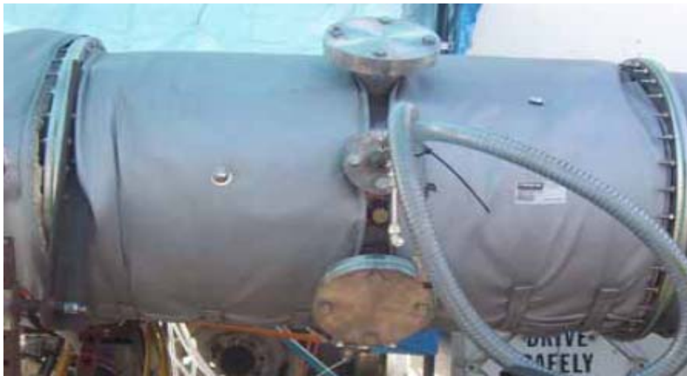
Figure 3.5 Ejector dilution sampling setup
